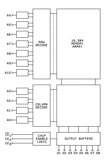
FIGURE 3. Functional block diagrams.
