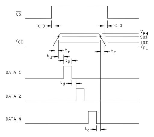
FIGURE 5J. Programming voltage waveforms during programming for circuit J.
