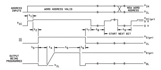
FIGURE 5H. <u>Programming voltage waveforms during programming for circuit H.</u>
