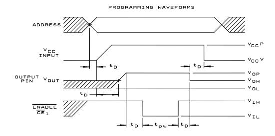
FIGURE 5B. Programming voltage waveforms during programming for circuit B.
